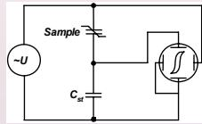
Samples are prepared by Pulsed Laser Deposition, and subsequent masking with ohmic Pt back and front contacts. Electric and electrooptic ellipsometry measurements were performed on contacts and near contacts, respectively.
