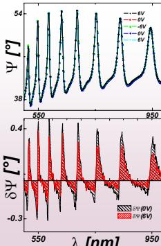
Electrooptic ellipsometry difference spectra reveal effective (overall structure) index and thickness change hysteresis indicative for polarization coupling, and concordant with asymmetric electric and polarization hysteresis switching behavior. From best-fit model analysis of Sawyer-Tower circuit measurements we estimate the spontaneous polarization in the ZnO layer.
