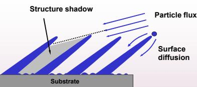
The incoming particle flux at glancing angle causes self-organized column growth due to preferential growth of nucleation sites, structure shadowing, and limited surface adatom movement.
