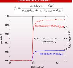
The graph above displays the calculated thickness of synperonic film over time as calculated from QCM data ( $q_{\rm CCM}$ ) and SE data ( $d_{\rm SE}$ ). Also shown is the variation of porosity ( $f_{\nu}$ ) over time as the film is formed. Knowing the porosity yields an insight to the amount of trapped water in the organic thin film
