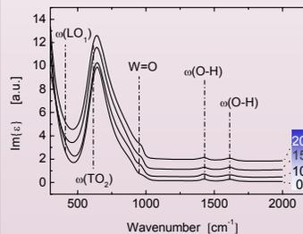
**Right:** Bands of total reflection (TO-LO phonon bands) for the tungsten oxide films versus charge intercalation density. **The stretching W-O-W mode is losing polarity upon intercalation, while the double-bond modes gain strength. This is indicative for intercalation-induced bond reformation.**
