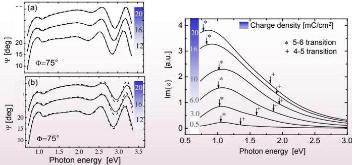
Experiment and best-match model calculated ellipsometry data in the VIS-UV range at various intercalation states. (a) Gaussian and Lorentz, and (b) single-Lorentz lineshape approximation for the polaron contribution. The double oscillator model describes precisely the experimental data.
