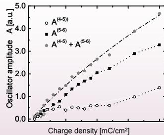
Oscillator amplitude parameters in dependence of the charge density for the 4-5 and 5-6 polaron transition. The sum of the oscillator amplitude follows an asymptotic saturation behavior characteristic from polaron hopping.
