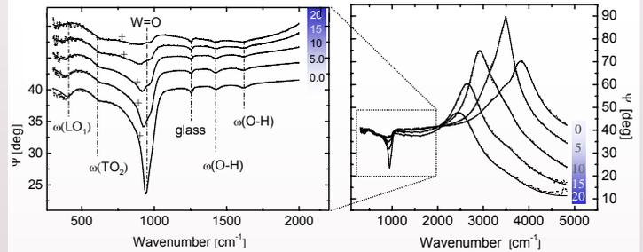
Experiment and best-match model ellipsometry data (Ψ) in the MIR range of tungsten oxide thin films with various intercalated charge densities. The phonon modes of interest for structural information are found below 2000 cm<sup>-1</sup>. The cross symbols denote the position of the LO<sub>2</sub> mode.
