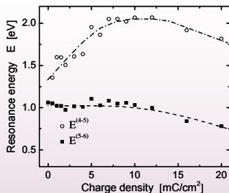
Oscillator resonance energy parameters of the 4-5 and 5-6 polaron transition. For charge densities higher than 10 mC/cm<sup>2</sup>, the hopping energy is reduced with increasing charge density. The dotted lines are a guide to the eye
