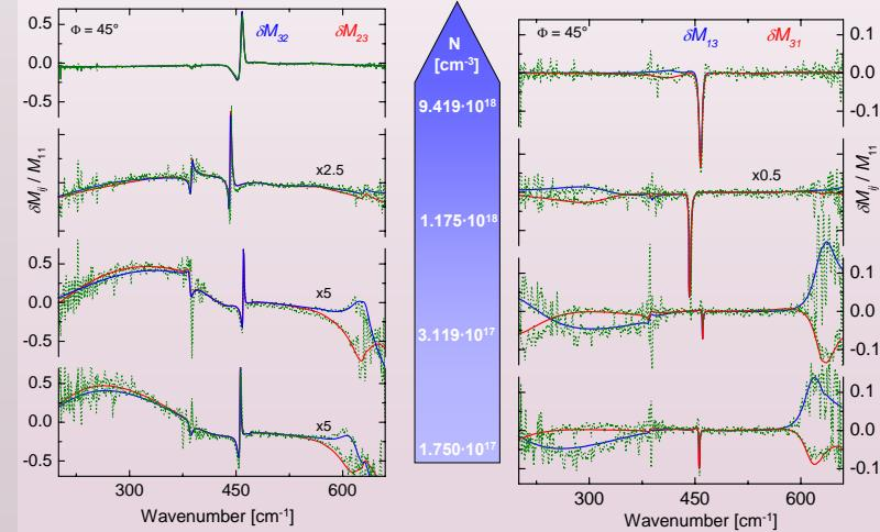
The spectra above are differences between Mueller matrix data (chiral elements  $M_{13}, M_{31}, M_{23}$ , and  $M_{33}$ ) measured magnetic fields of +4.5T and -4.5T. The non-chiral elements  $M_{12}, M_{21}, M_{22}$ , and  $M_{32}$  vanish. Vertical solid and dashed lines within the Standard Ellipsometry spectra indicate the TO and LO mode frequencies, of the InN film and the sapphire substrate.
