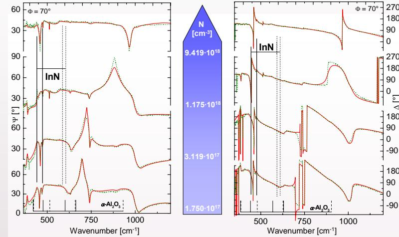
Zero-Field Standard Ellipsometry spectra reveal thickness, phonon mode frequency and broadening parameters, static dielectric constants, plasma frequency and plasma broadening parameters of InN and GaN layers upon model layer calculations
