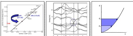
Experimental and theoretical evidence for  $E_g(\text{InN}) \sim 0.7 \text{ eV}$
